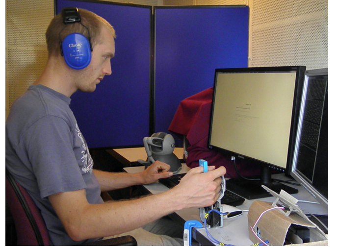
(a) Experimental protocol including the ANGEL device. The user places his thumb in the device and perceives a pressure on it. He wears hearing protection to avoid hearing the actuator of the device.
